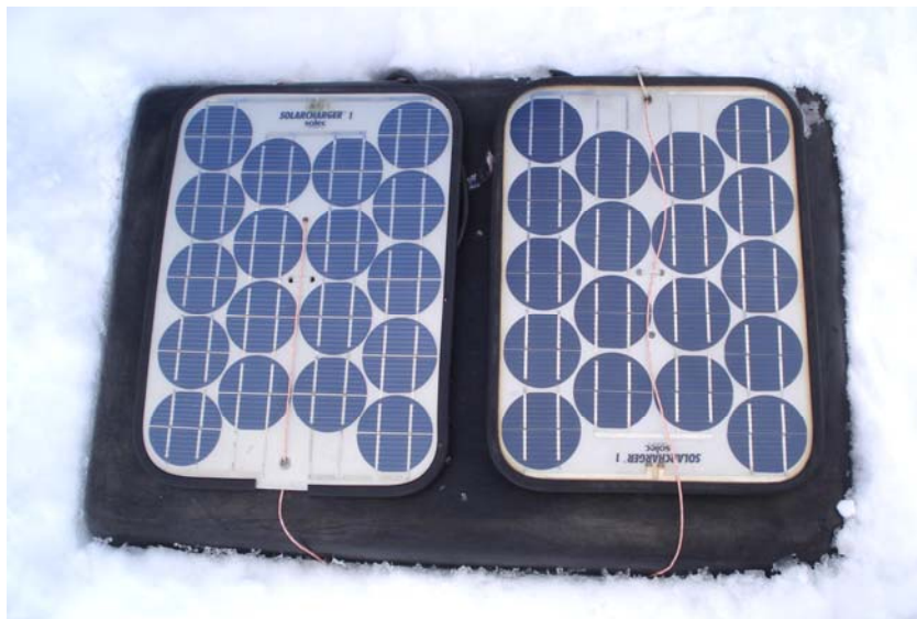
Fig. 6 Two Soltec-M1136 solar panels for powering the battery chargers of the Motorola GP328 radios
